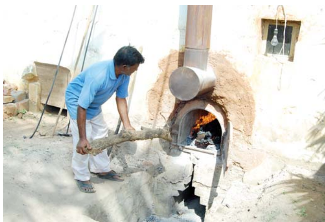
Ventury furnace to reduce the fuel usage
